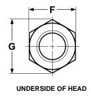
‡Length of a machine bolt is measured from the underhead bearing surface to the extreme end of the bolt.
